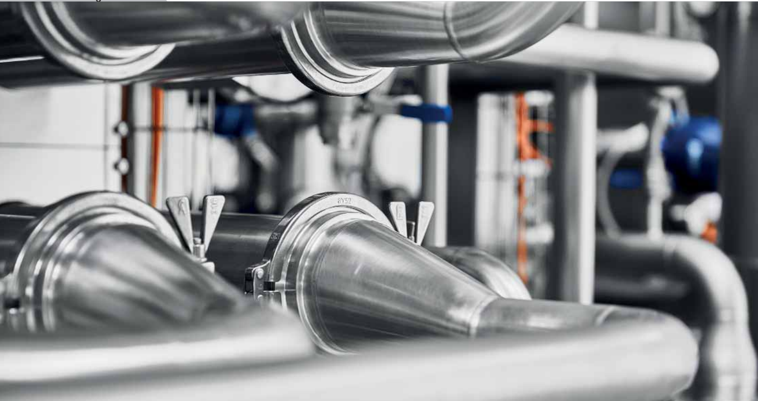
Corrugated tube heat exchangers such as the HRS MI Series, are ideal for pasteurising liquid egg and other egg products
