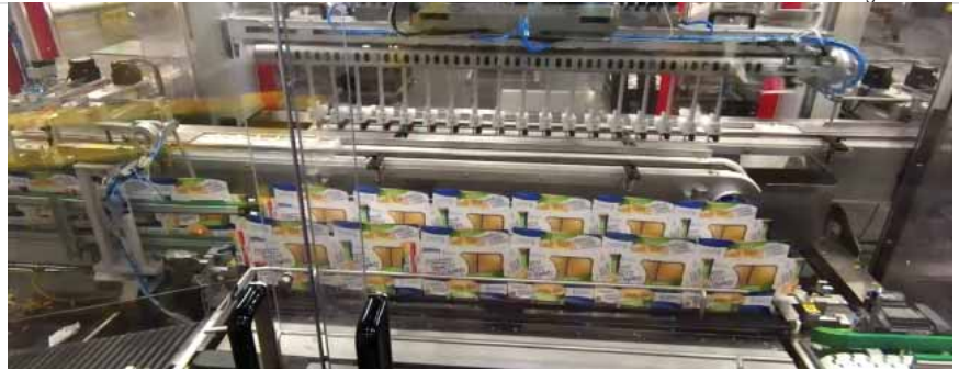
The IER 030 topper places 400 bags per minute into the secondary packaging. | (Image: Sacmi)
